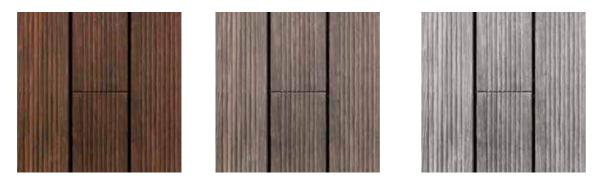
Gradual greying of Bamboo X-treme<sup>®</sup> over time: new, non-weathered decking (left), after 3-6 months of weathering (middle) and after 18 months of weathering (right).
