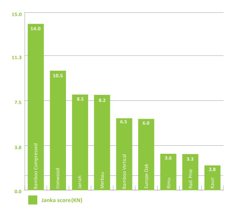
The hardness of wood is calculated by the Janka hardness test, which measures the force required to embed an 11.28 mm steel ball into wood to half the ball's diameter. It determines the ability of a type of wood to with-stand denting and wear. The higher the Janka rating, the harder the wood.
