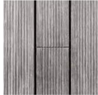
Gradual greying of Bamboo X-treme® over time: new, non-weathered decking (left), after 3-6 months of weathering (middle) and after 18 months of weathering (right).
