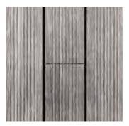
Gradual greying of Bamboo X-treme<sup>®</sup> over time: new, non-weathered decking (left), after 3-6 months of weathering (middle) and after 18 months of weathering (right) - without oiling.
