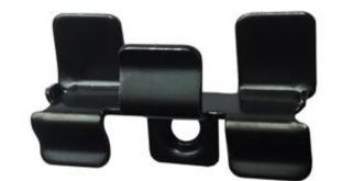
With correct joist set-up, bamboo X-treme decking can be quickly installed using the powder-coated stainless steel clip and screw fixings supplied (for "invisible" fixing – no unsightly nails or screws visible).
